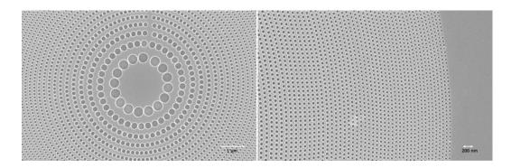
Figure 2 SEM image of atom sieve fabricated using electron beam lithography: SEM image of atom sieve prior to etching.
